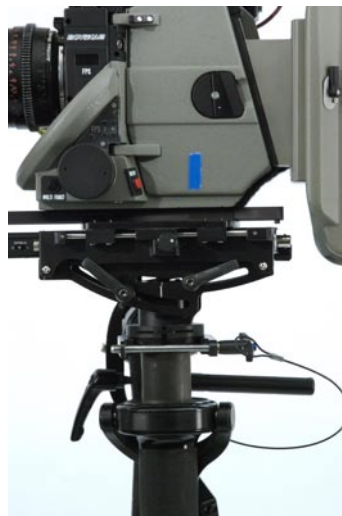
Camera c.g. .75" behind center post – fore-aft.
