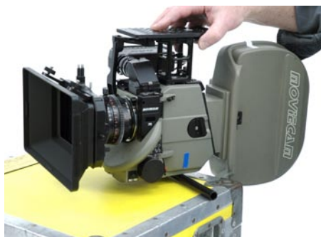
Finding the camera's fore-aft center of gravity.
