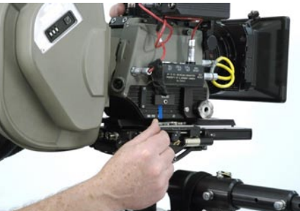
Closing the locking lever.
