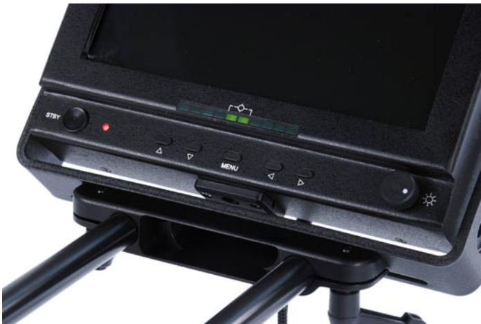
Artificial Horizon and menu navigation controls
